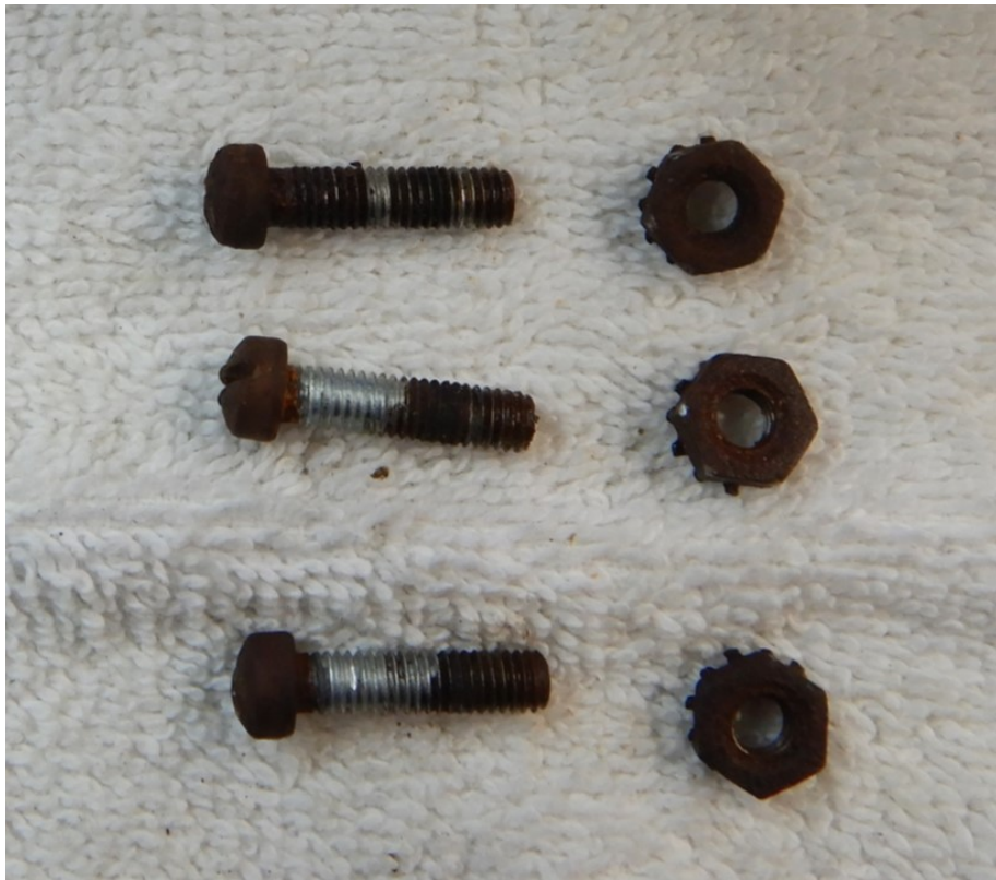
Figure 5: Badly rusted metal fasteners – These aren't the worst ones
