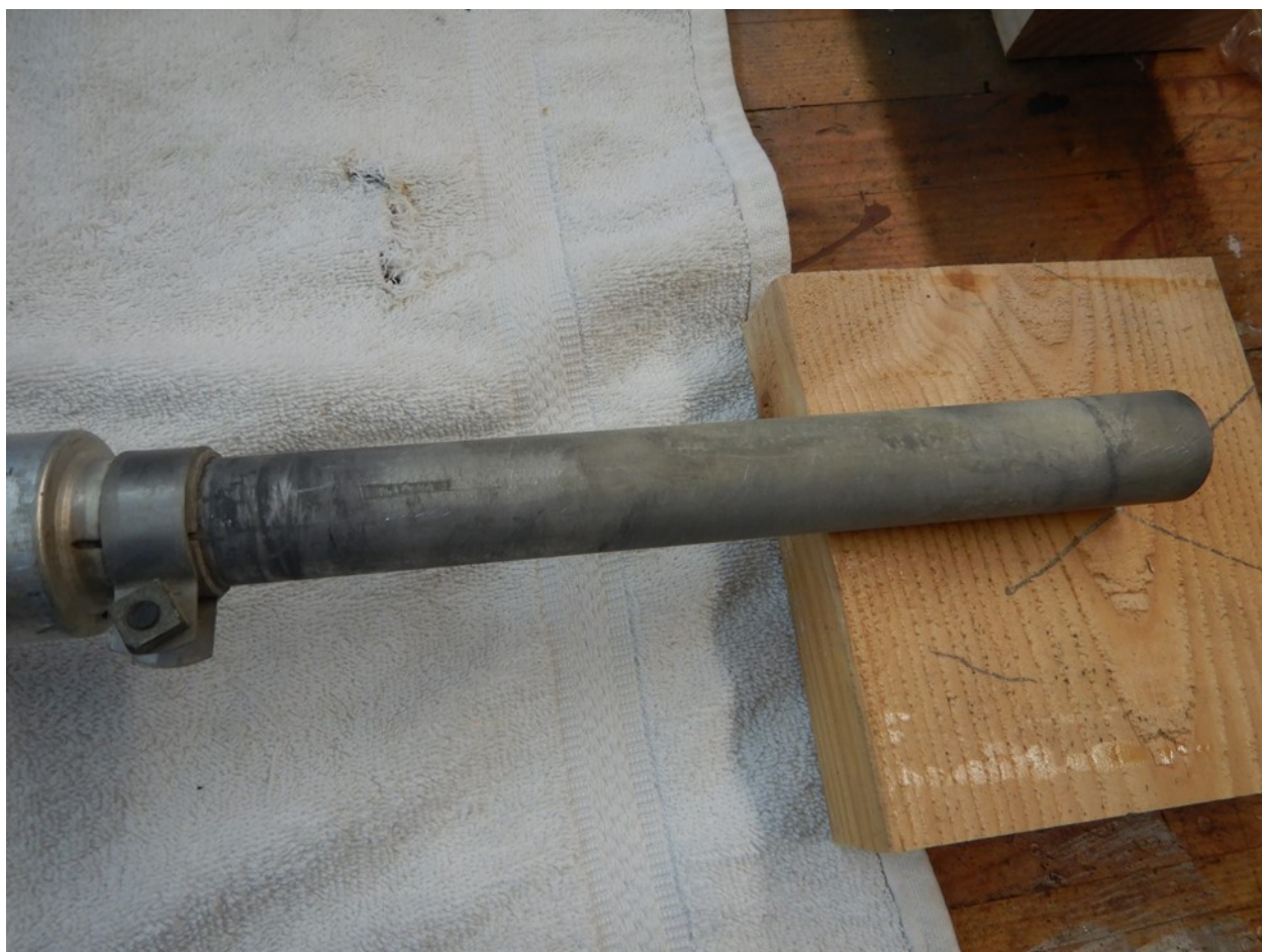
Figure 1: Extreme Corrosion at element connection points
