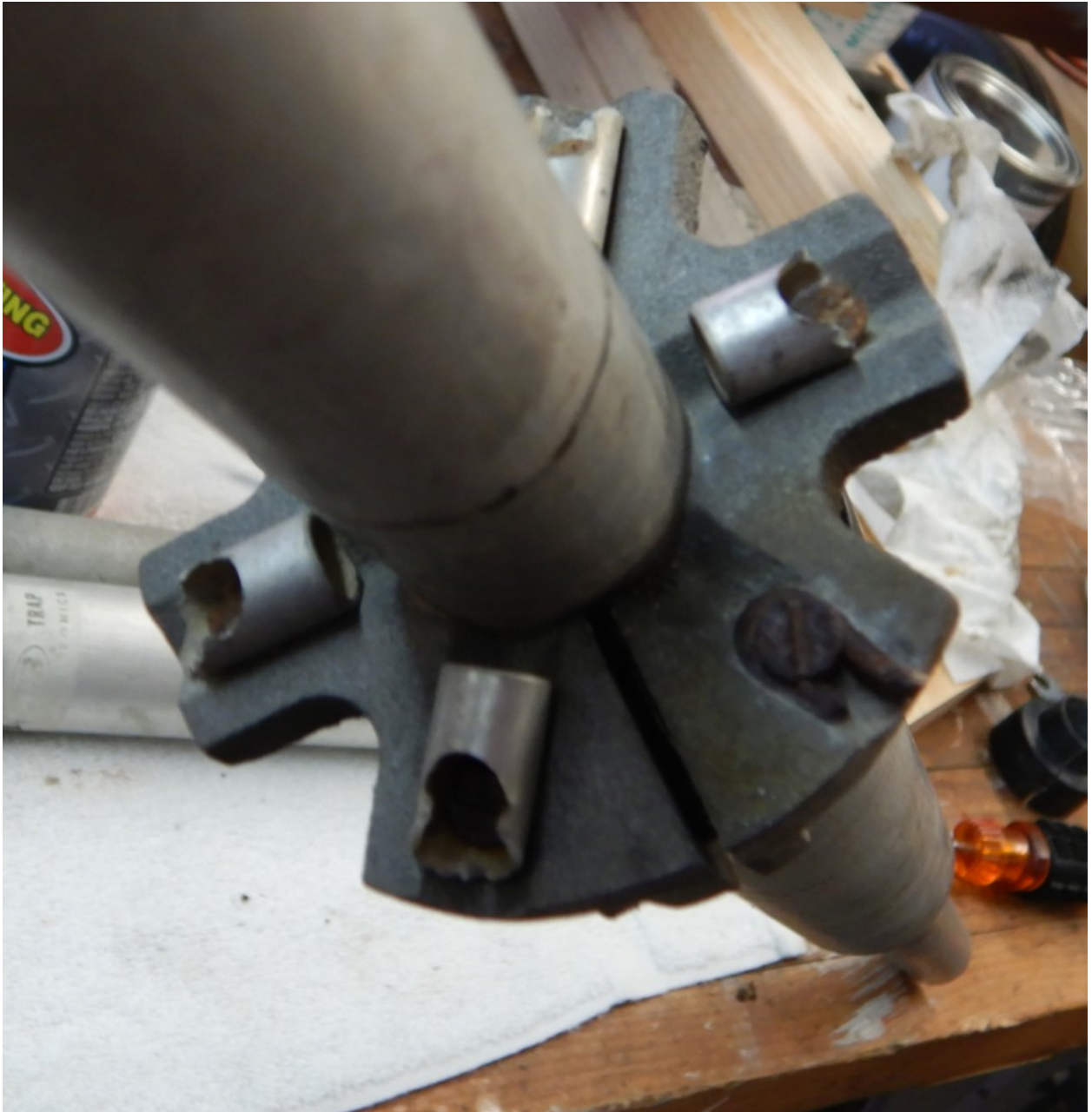
Figure 4: A view of the spider hub. The slots in the screws have all but rusted away!
