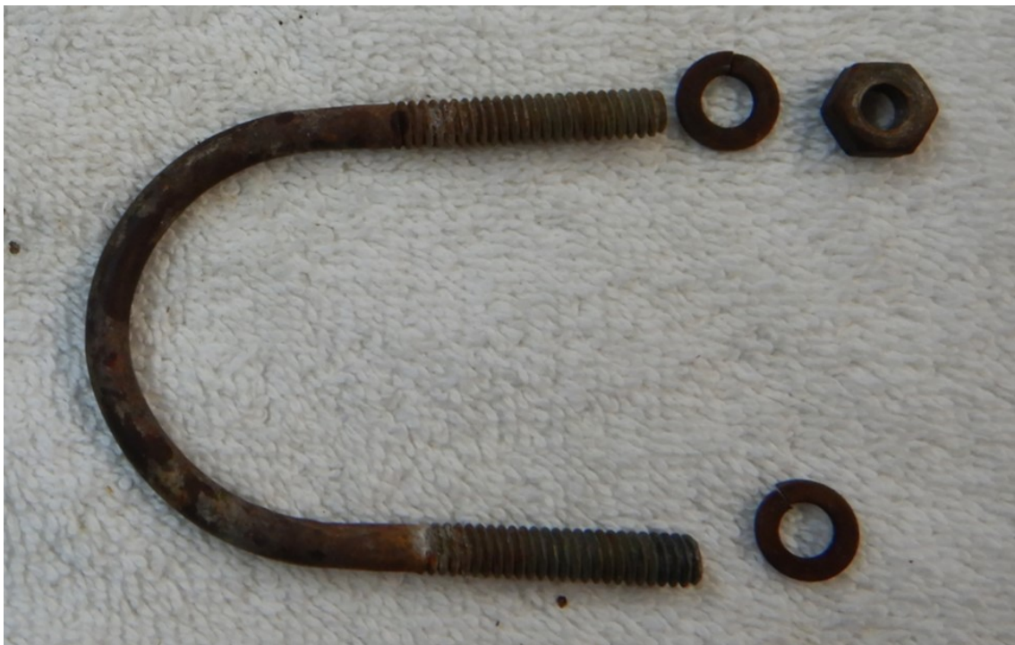
Figure 3: Rusted U Bolts. I hate to think how many of these I've seen twist off because the bolts were so baldy rusted
