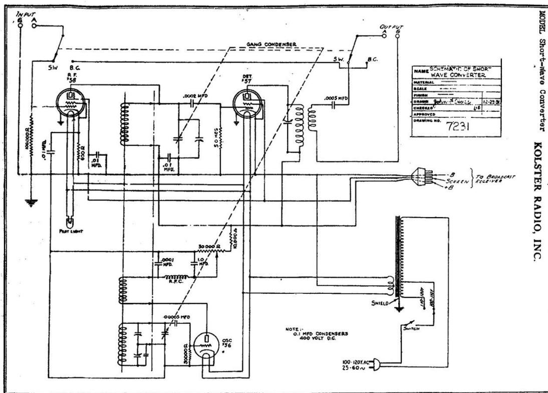
This three tube converter made the radio capable of operating on some of the lower frequency amateur bands. The radio was built for amplitude modulated (AM) reception for voice. I do not see a beat frequency oscillator for code reception.
