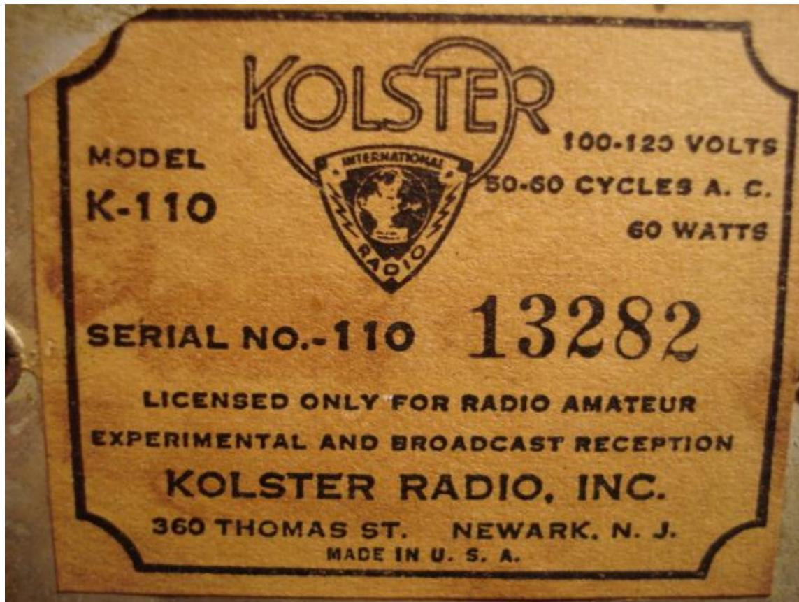
Notice the reference to Radio Amateur use. The K-110 was a broadcast only receiver, but had a jack on the rear chassis that accepted input from a shortwave converter.
