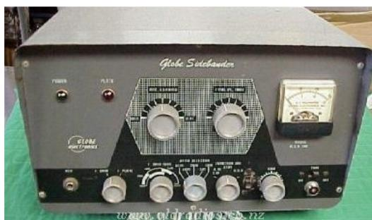
DSB 100 Double-sideband transmitter. It put out 50 watts on CW, 40 on AM and 100 on DSB no carrier.
