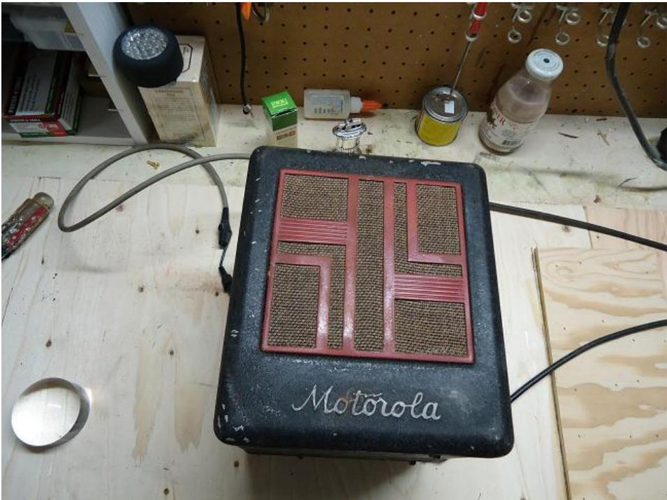
This is the "control head" for the radio. This mounted on the steering column and the controls were connected to the radio chassis via steel cables, much like a speedometer cable.
