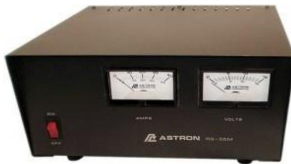
After removing the cover, I vacuumed all the dust out of the supply. The RS-35M wasn't very dirty, but even so, getting the dirt out of a piece of equipment is probably the first thing you'll want to do when performing preventive maintenance. Dirt impedes air flow. That can lead to higher operating temperatures, and as the lab manager that I interviewed for my blog post said, "Heat kills."
