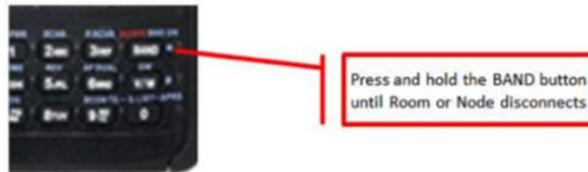
Figure 90 FT1D and FT1XD Disconnect method
