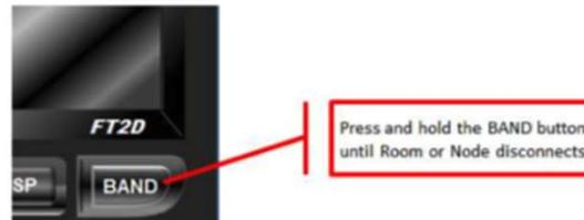
Figure 91 FT2D Disconnect methods
