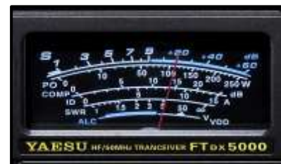
Figure 1: S-Meter in the Yaesu FTDX-5000. It's showing an incoming signal of 20dB over S-9.
