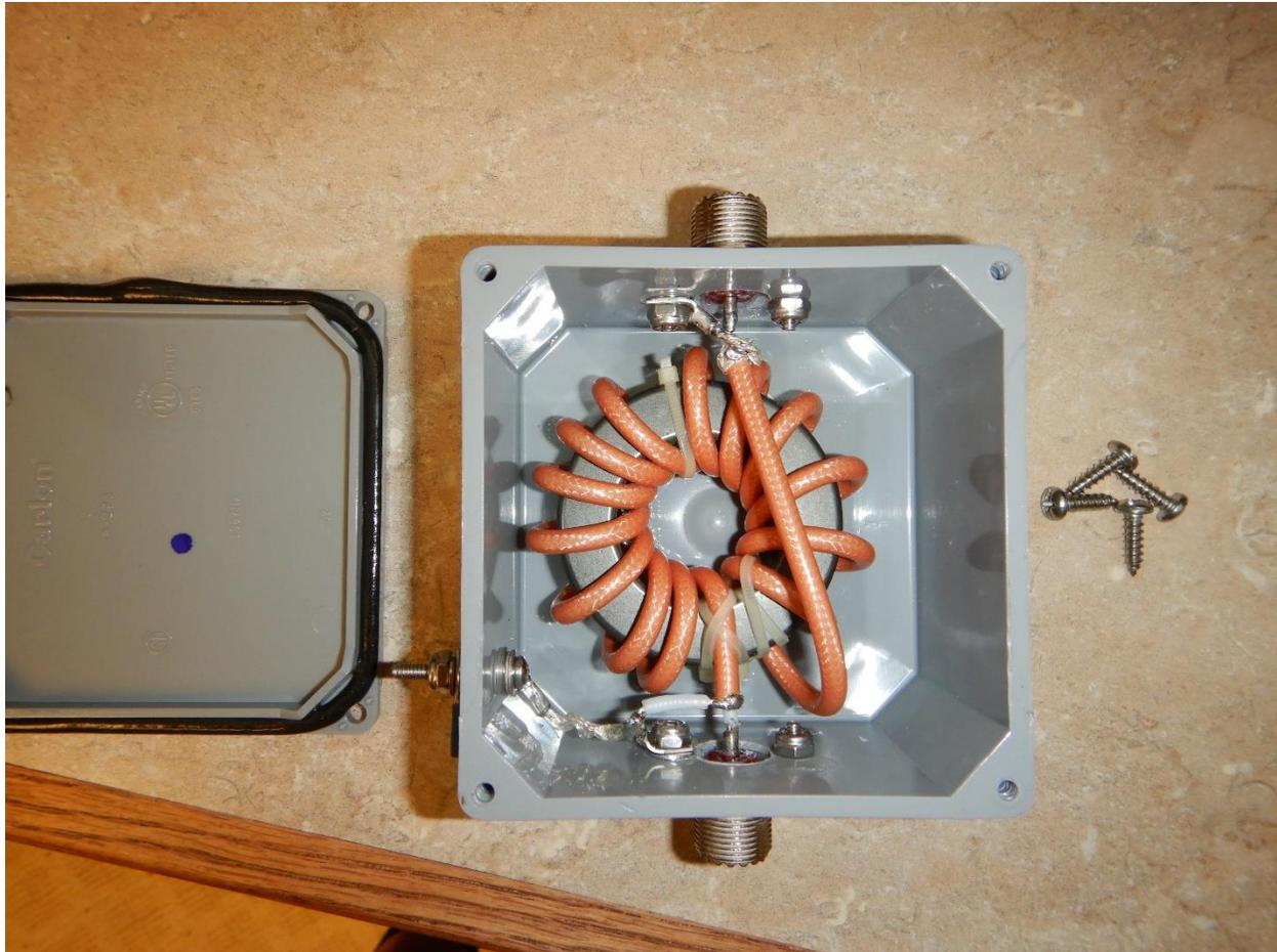
Figure 5: Common Mode Choke made using RG-400
