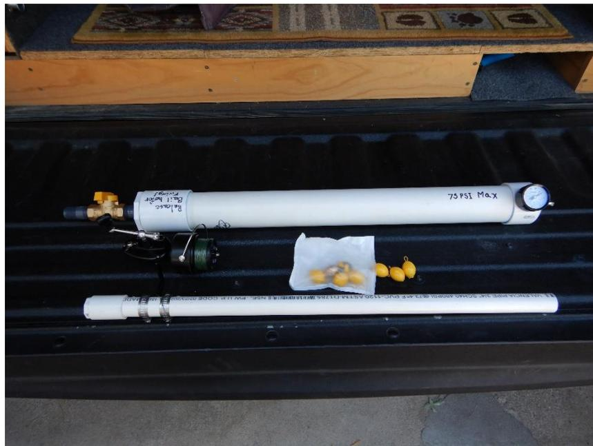
Figure 1: The Air Powered Antenna Canon
