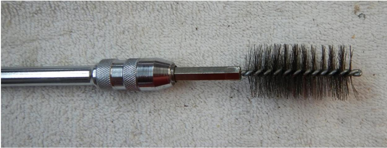
*Figure 9: Tubing Cleaner attachment*
