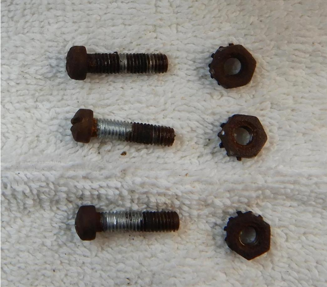
*Figure 5: Badly rusted metal fasteners – These aren't the worst ones*
