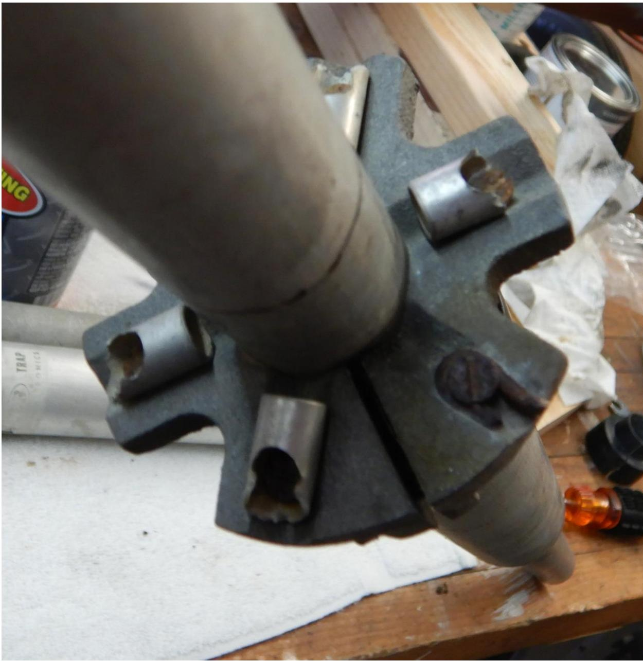
*Figure 4: A view of the spider hub. The slots in the screws have all but rusted away!*
