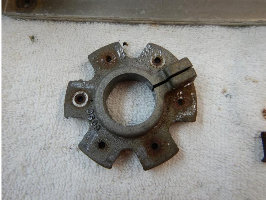
*Figure 7: The spider hub before restoration*
