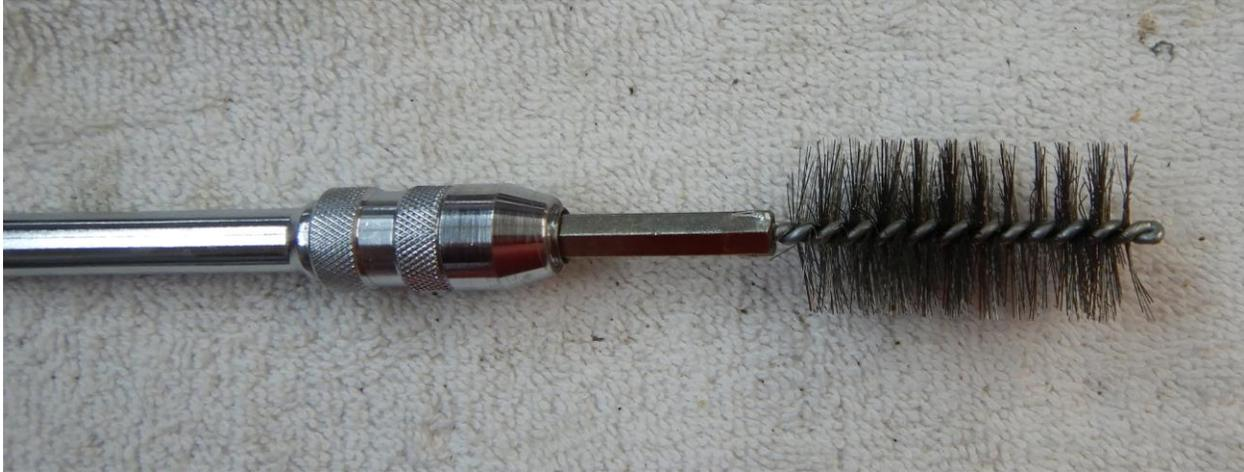
*Figure 9: Tubing Cleaner attachment*
