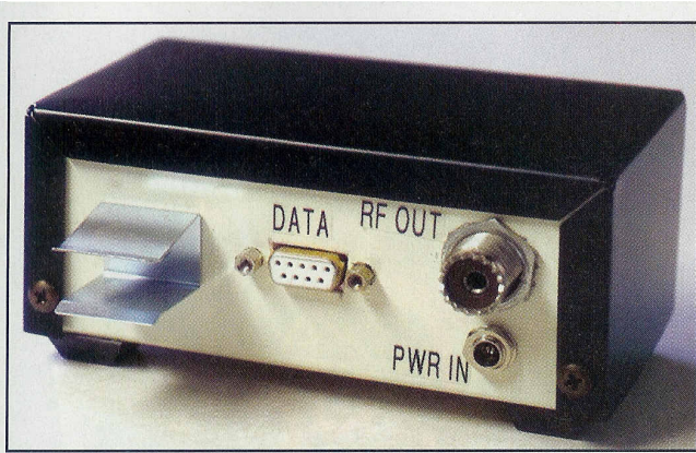
Photo B- Rear view of the beacon transmitter. The 9-volt battery clip permits portable operation. The DB-9 data port is for hooking up a computer to program your call sign and other options.
