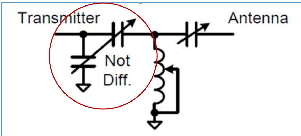
Figure 14: Lew McCoy WIICP, *Ultimate Transmatch* (1970). Note the Split-Stator circled in red.
