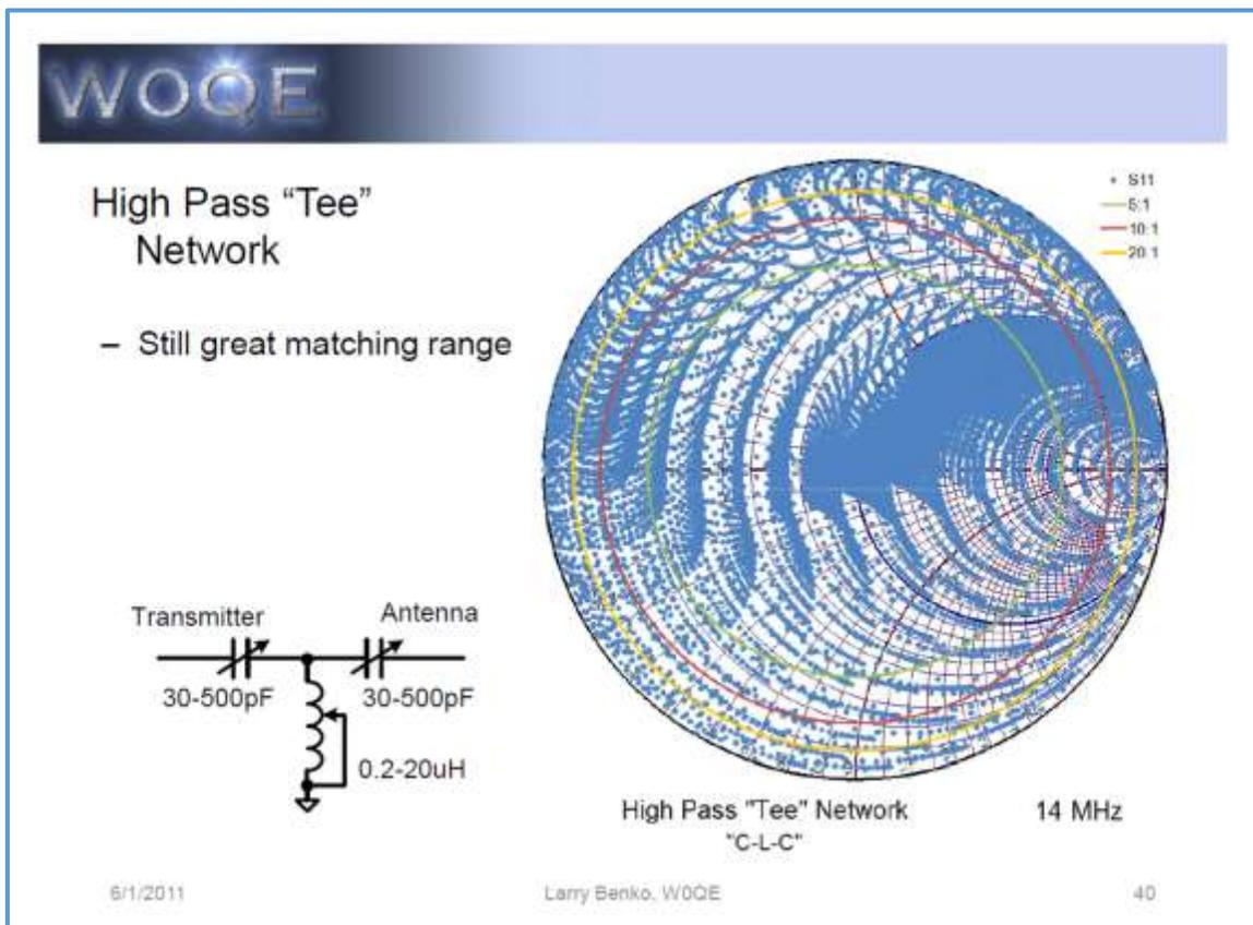
Figure 12: The High Pass "T" Network for 20 Meters
