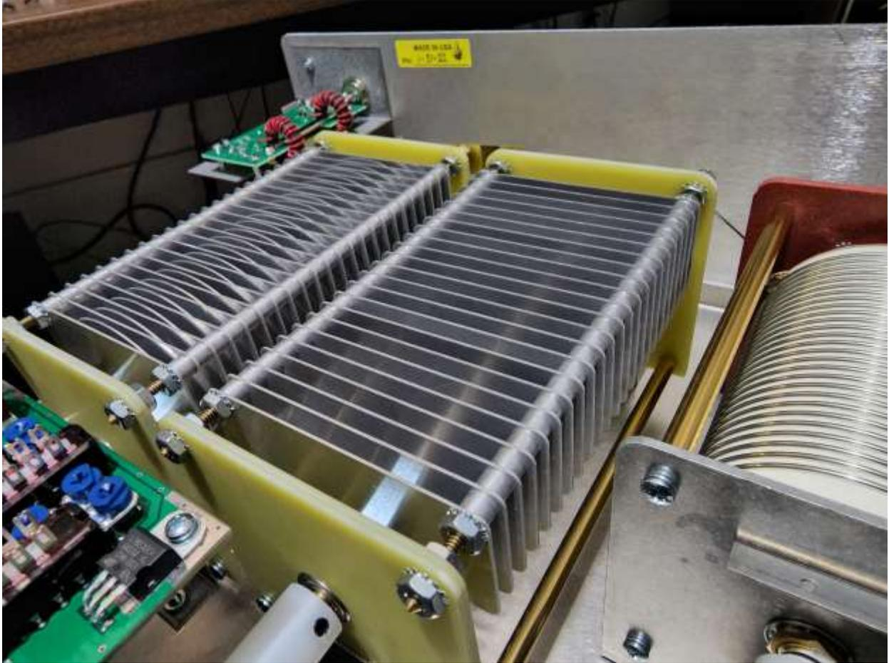
*Figure 86: Palstar AT2K variable capacitors*
