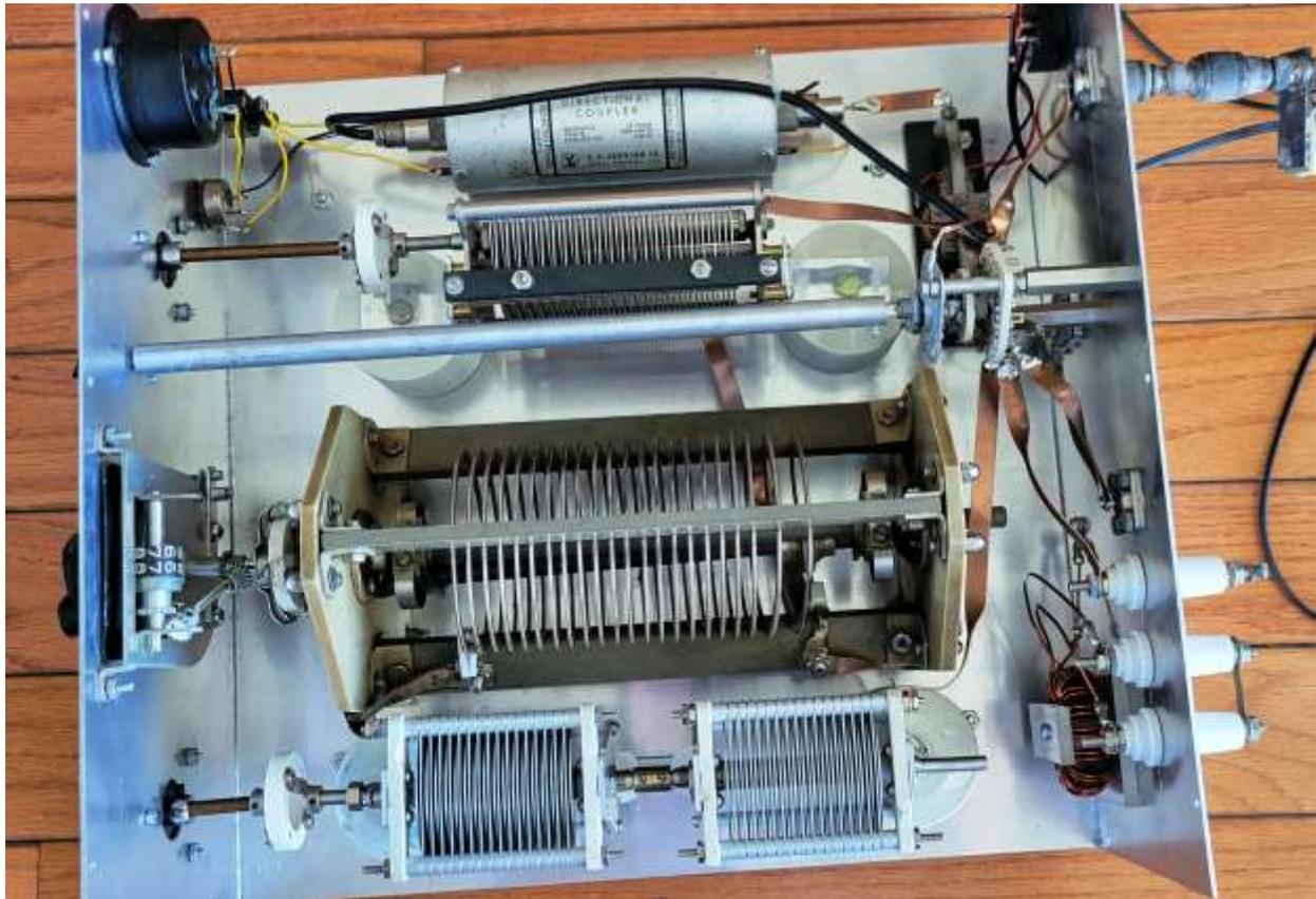
Figure 32: KBOES Home Brew Ultimate Transmatch. Note the massive inductor and the use of copper strips rather than round copper wire. This is a very well made tuner, one of the best I have seen.
