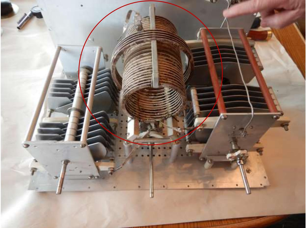
*Figure 60: The inductors are tarnished due to the fact they were silver plated. No expense was spared in the building of these fine old tuners. Also note the inductor in an inductor. This is why this tuner is referred as inductor coupled.*
