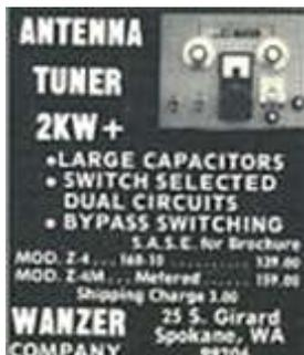
It came in two models, one with meters (Z-4M) and one without meters (Z-4). Top of the line model included a relative fwd/ref output meter. Had an "in-out" switch and a switch to change from a "PI" configuration to a "T" configuration. It utilizes two 750pf heavy duty variable capacitors and a 28uh plated roller inductor with a turn counter. The WaZer Match covered 1.8 to 30 MHz and could handle full legal limit. Physically it was a fairly small at 9x8x5.
