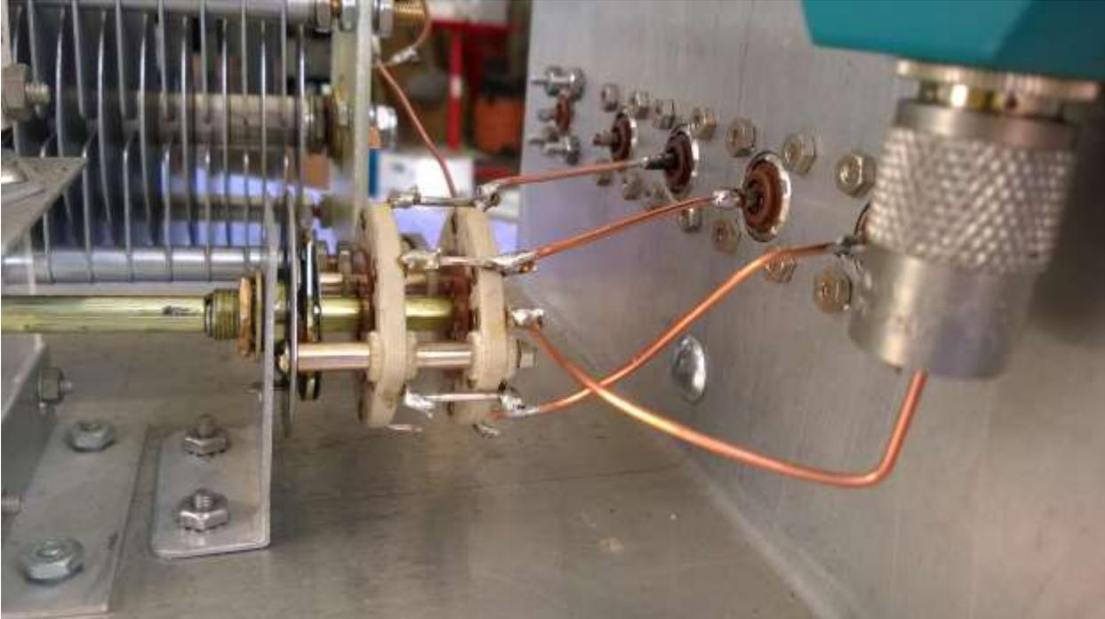
*Figure 71: WB7RLX Differential Tuner - Rotary Switch. My key goal in wiring the components was to keep the leads as short as possible in an effort to minimize loss and stray capacitance. I will eventually replace the rotary switch with a higher quality switch. This switch is out of the MFJ-986 Tuner. The contact surface area is pretty small when compared to higher quality switches.*
