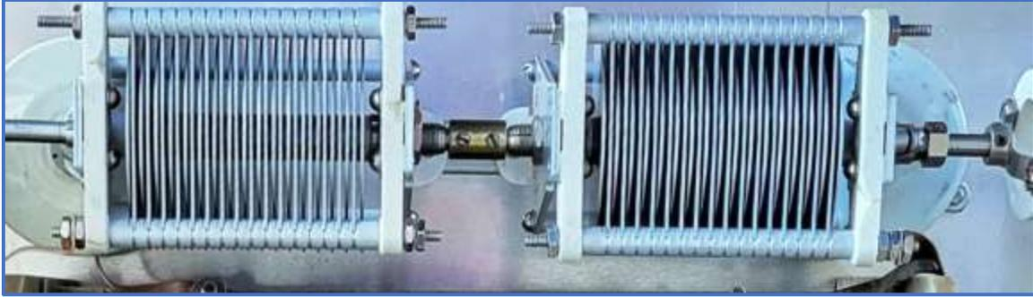
*Figure 15: Variable Split Stator - Basically a split stator is two capacitors sharing a single shaft. You can wire the device to be two independent devices or connect the two capacitors together in series to increase the range of the device.*
