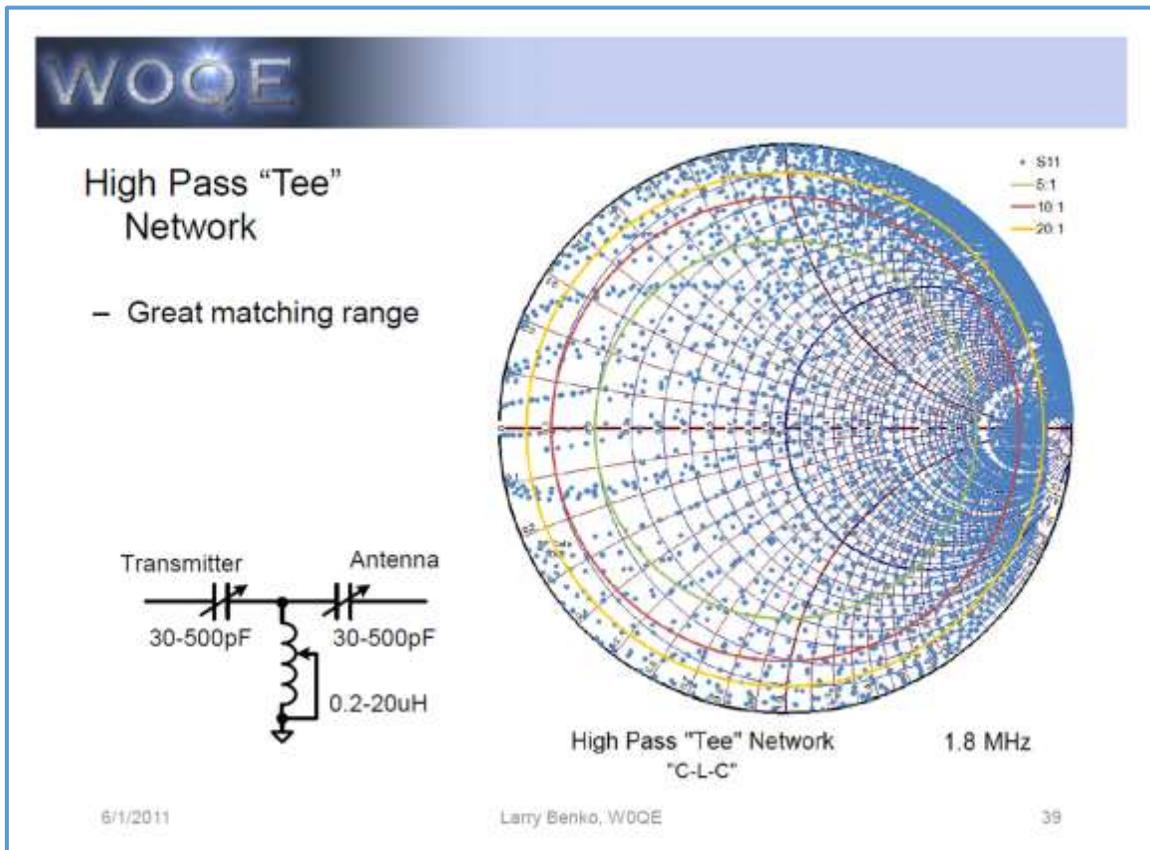
Figure 13: The High Pass "T" Network for 160 Meters
