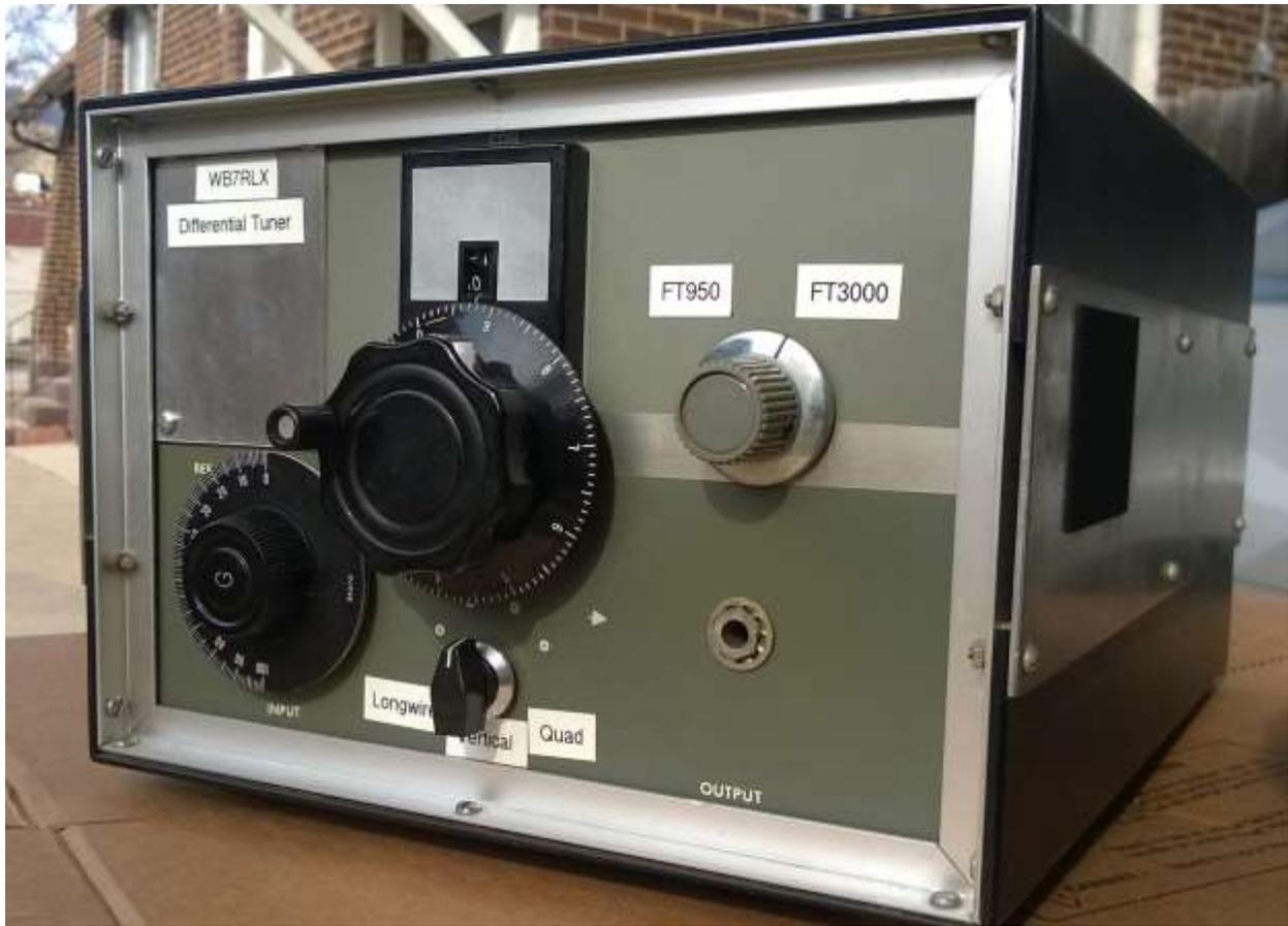
*Figure 66: WB7RLX Differential Tuner – Note the unused hole in the front. I'm going to mount a propagation compensator in the unit and locate the control switch there. A note on the six position antenna selector switch: When the switch is pointing above horizontal, as it is in the picture, the tuner is engaged. If the arrow is pointing below the horizontal then the tuner is disengaged.*
