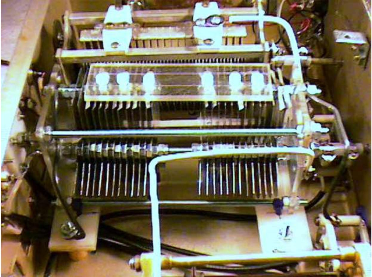
*Figure 36: Hammack SPC Tuner – Homemade Variable Capacitor*
