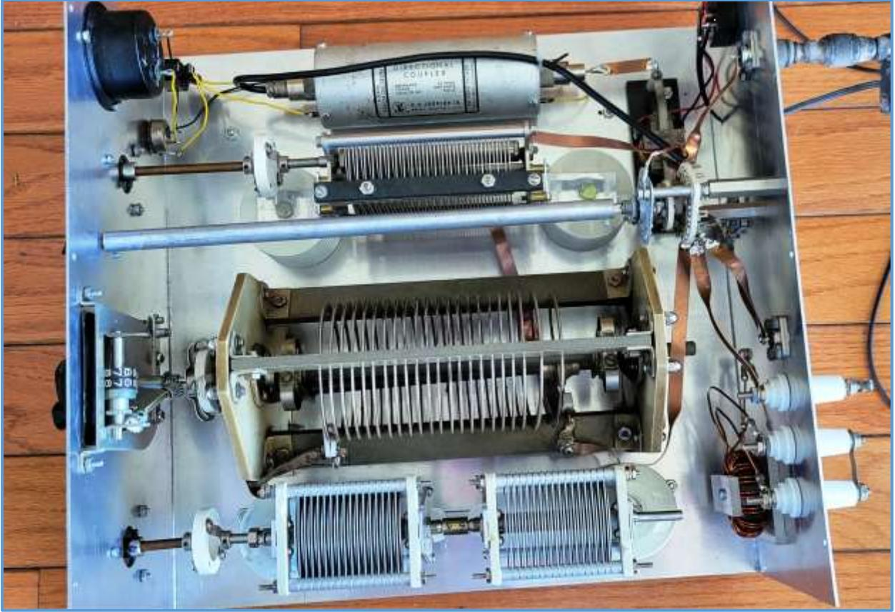
Figure 17: Homebrew Ultimate Transmatch built by John Burger KB0ES. This tuner was built in 1977. Note the use of the interconnecting copper straps and the high quality rotary switch.
