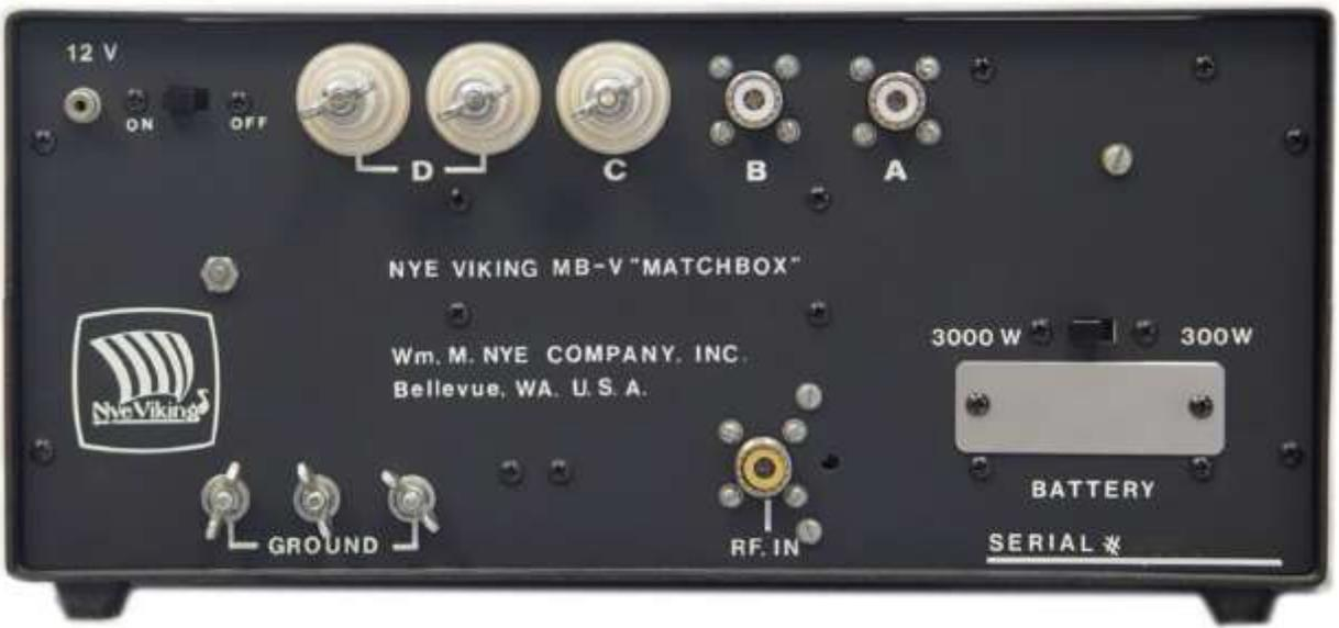
Figure 44: Nye Viking 3KW Tuner - Rear view
