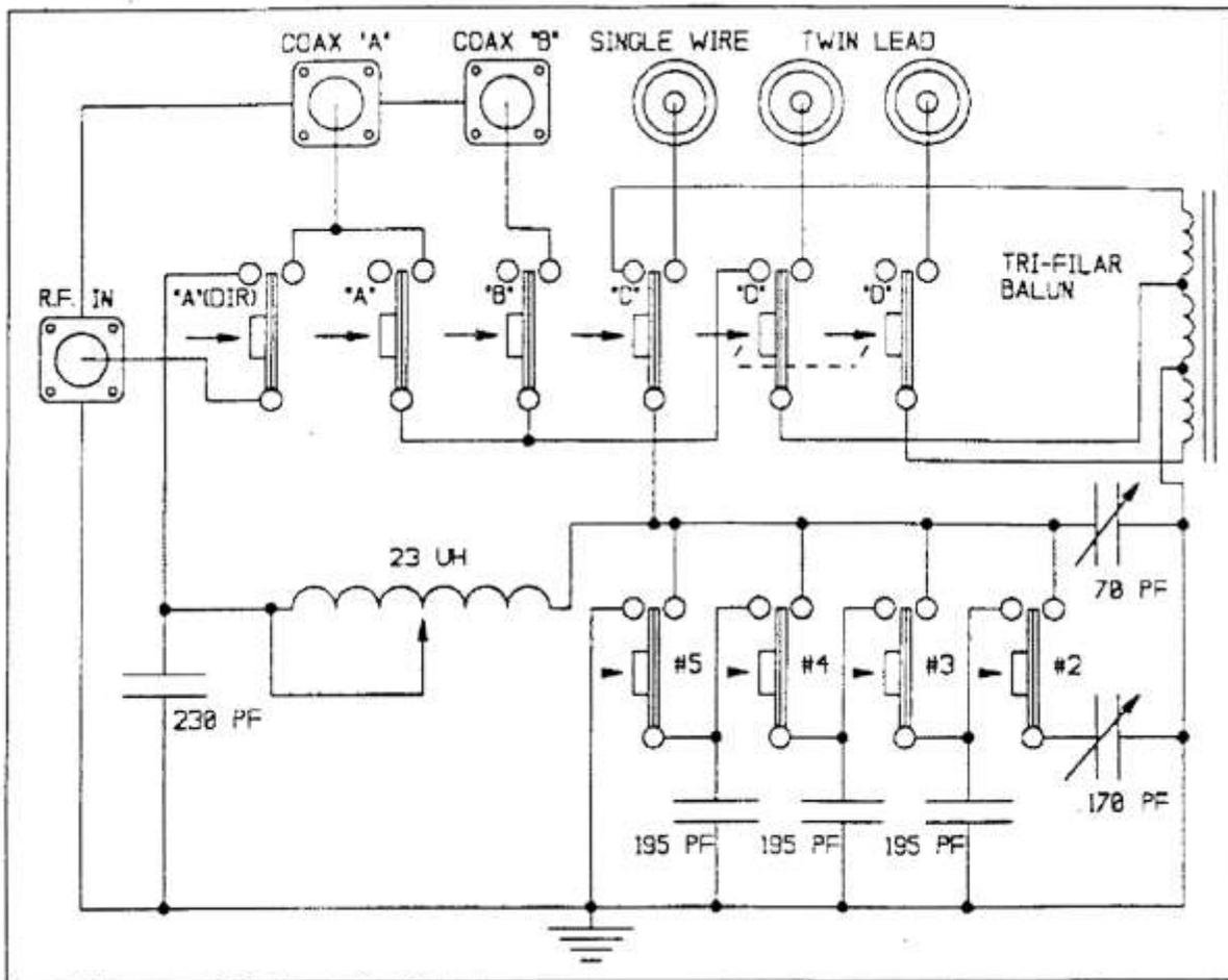
Figure 42: Schematic of the Nye Viking MB-V-A-3KW Tuner
