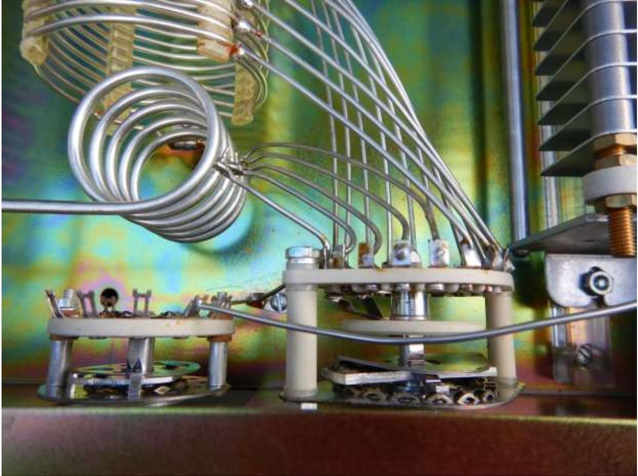
*Figure 41: Denron MT-2000A. A close look at the robust rotary switch.*
