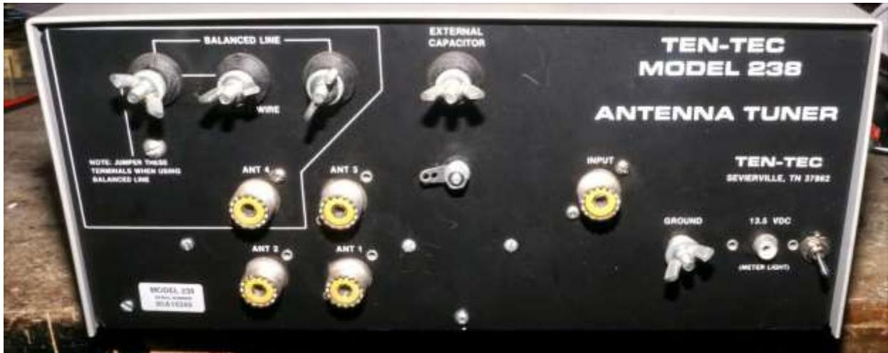
Figure 49: Ten Tec Model 238 - Rear view
