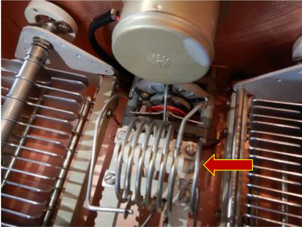
*Figure 75: James Millen 92200 Ultimate Transmatch - Note the small loop to the right of the small induction coil. That coil is the sensor for an oscilloscope. The socket for the oscilloscope is on the rear panel.*
