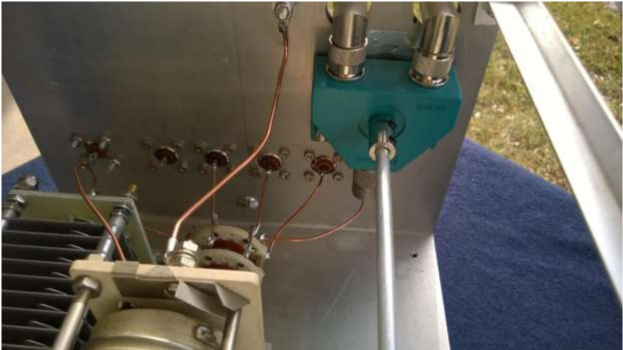
Figure 70: WB7RLX Differential Tuner - looking toward the antenna switch. Note the two ports on the left are not used.
