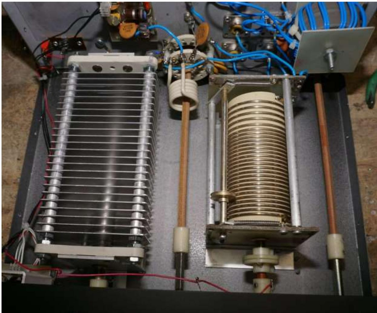
Figure 50: Ten Tec Model 238 - Interior view
