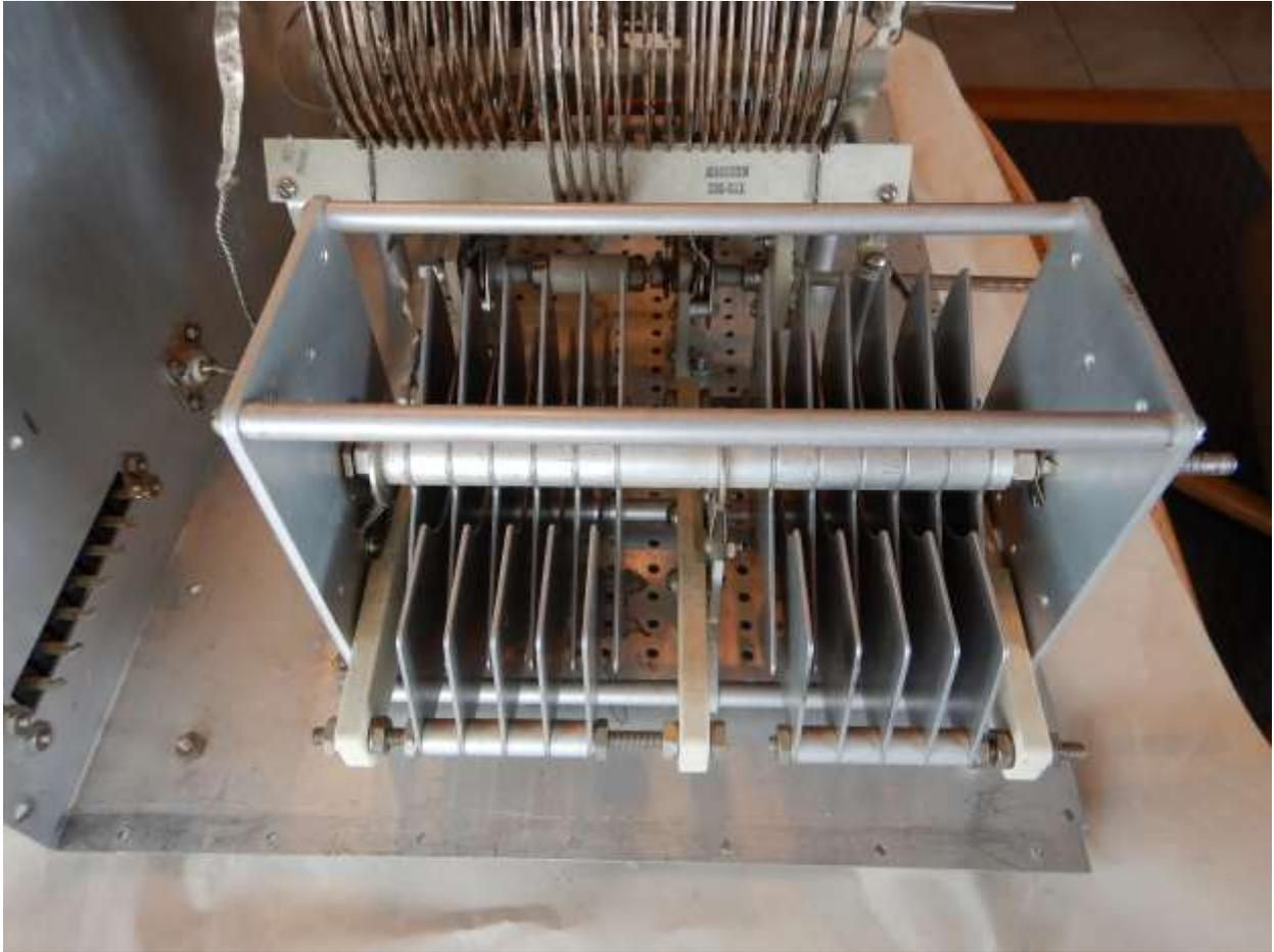
*Figure 62: KW Johnson Matchbox - The other variable capacitor*
