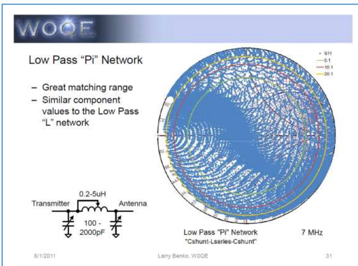
Figure 8: The Low Pass "Pi" Network
