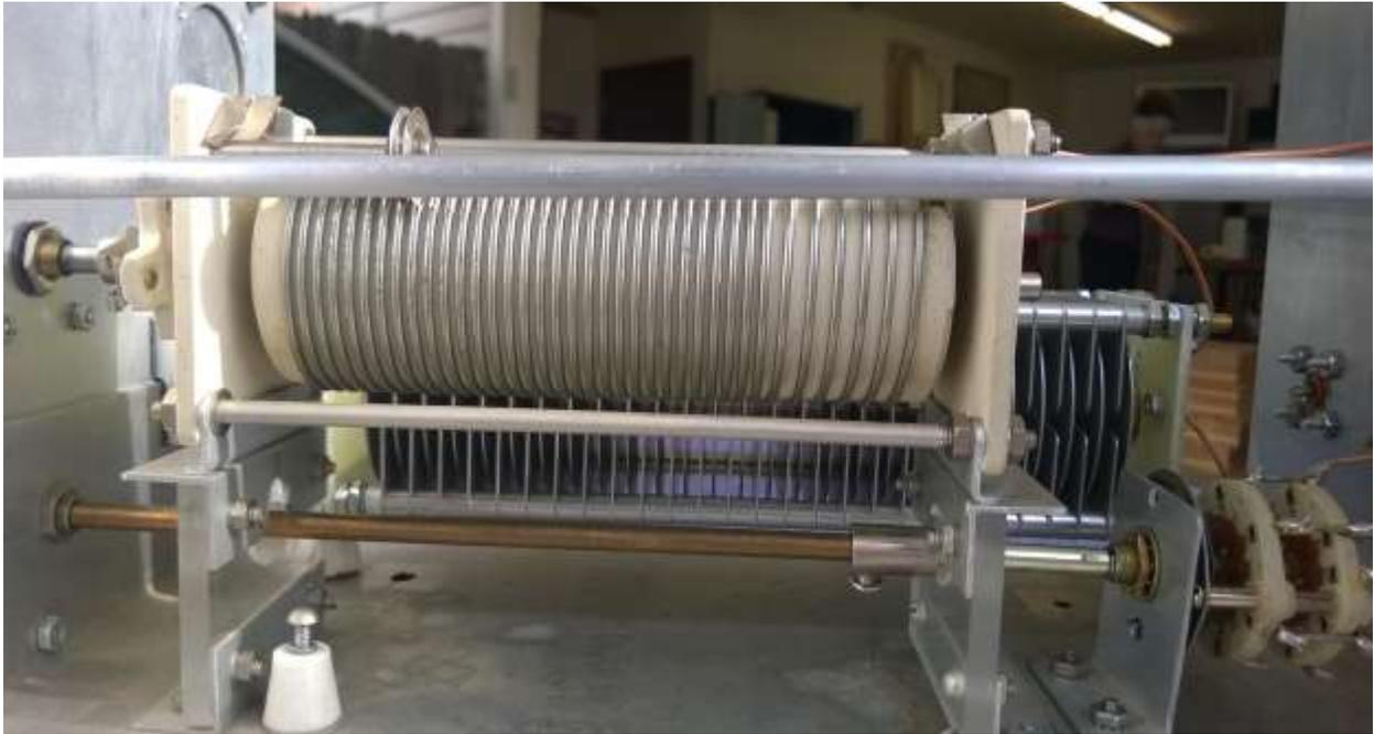
Figure 69: WB7RLX Differential Tuner – Inside. This is a good view of the roller inductor. Note also that I replaced the brass shaft going to the rotary switch and the aluminum shaft going to the input switch with fiberglass rods. I wanted to minimize any potential for stray capacitance.
