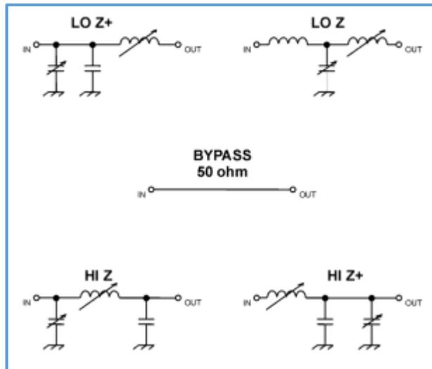
Figure 47: Ten Tec Model 238 tuner configuration options
