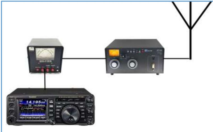
*Figure 28: Typical Station Using an External Tuner*
