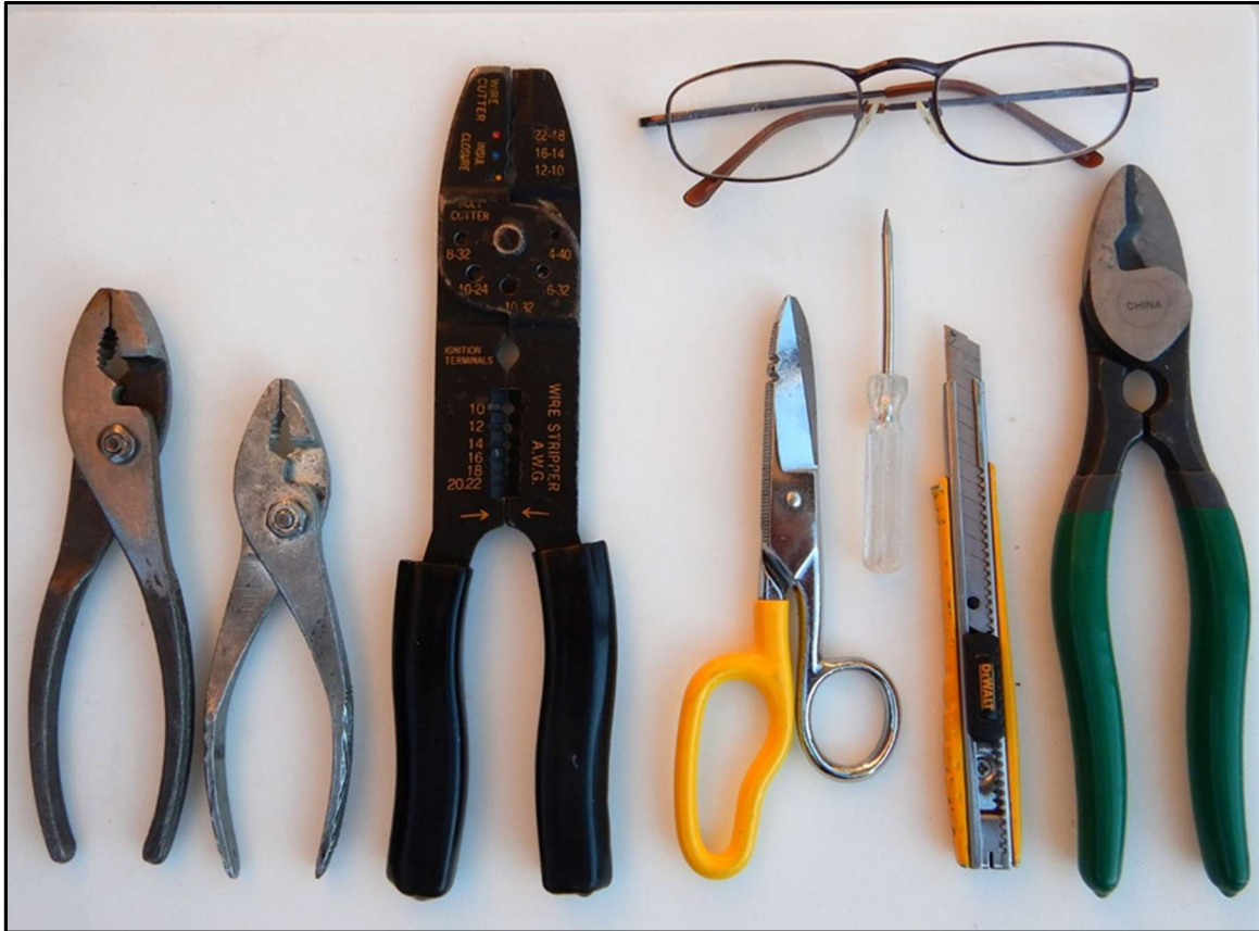
Figure 15: This is my tool tray when mounting connectors. Not shown is a small vice, a file, larger cable cutters, crimping tool, soldering station, clip-on small heat sink for soldering.
