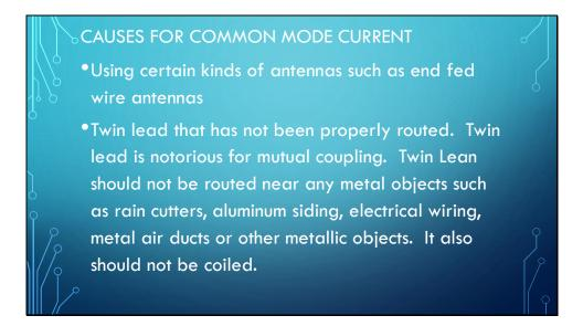
There's nothing wrong with using end fed antennas. They make a very good antenna when done properly. What that means you must use an unun AND a choke to minimize the CMC. It also helps if you can ground the other side of the UNUN provided the ground lead won't be too long. The short length of wire going to ground will be a part of the antenna.
