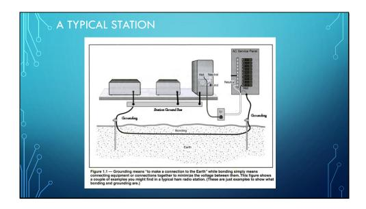
This slide shows an example of a properly connected station. Note the Electrical service and the ground rods and the station ground bus bar are all bonded together and that each piece of equipment is bonded to all the other equipment through the station ground bus. This configuration will also help to eliminate ground loops which are often responsible for humming on your signal when you transmit.
