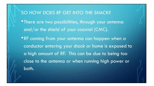
There is a way to tell where the RF is coming from. If you transmit into a dummy load and you don't see any of the effect you see when transmitting into your antenna then it's clear the RF is coming from either CMC or your antenna. If you still see the same effect when transmitting into the dummy load then it's likely that you have a bad bit of coax in the circuit or a faulty piece of equipment and/or you have a faulty ground or no ground at all.
