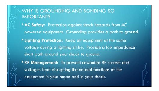
We are not going to cover AC Safety aspect in this presentation. Primary reason is AC Safety relies heavily on having a proper grounding system in place so we will focus on that. Also note that much of the wiring in your house has been done to address safety concerns. So we will focus our attention to Lighting Protection and RF Management.
