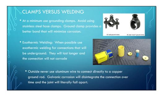
A note about galvanic corrosion. Over time galvanic action will result in the two metal components literally dissolving over time. Although in our dry Utah climate the problem is not near as bad in areas where there is exposure to salt water. There is a real problem for boaters on the Great Salt Lake. In your shack it's okay to connect copper and aluminum together as in the case of your station bus bar because the connection is not exposed to water or high humidly, but outdoors it a bad idea.
