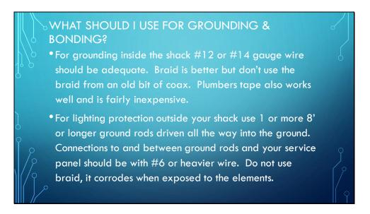
I have seen first hand examples of braid that has been use outside. Over time it corrodes. I would recommend you not use braid outside, instead use #6 or heaver copper wire or flat copper strips..
