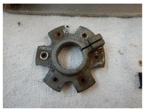
Figure 7: The spider hub before restoration
