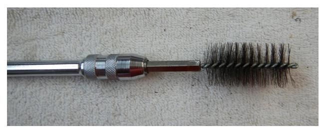
Figure 9: Tubing Cleaner attachment
