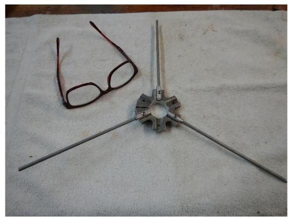
Figure 8: The new spider for 80 meters
