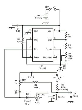
Figure 1—Schematic of the keyer/oscillator circuit. Radio Shack part numbers shown. Equivalent parts can be substituted.
