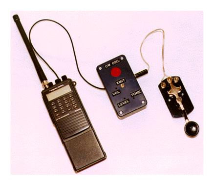
Title photo—Assembled, connected and ready to go! When you flip the transmit switch (labeled XMIT on this unit) the H-T goes into the transmit mode. As you work the key, the oscillator generates tones that are transmitted over the air.
