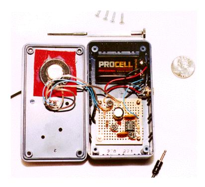
An interior view. The battery, speaker and circuit board fit within the case with room to spare.
