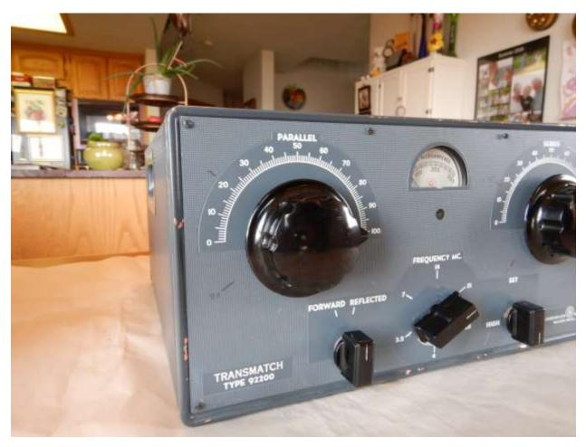
Figure 80: James Millen 92200 Ultimate Transmatch - Front left side. Note the copper where the paint has been chipped
