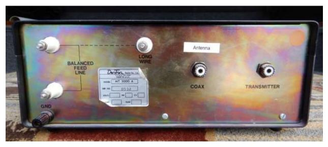
Figure 39: Dentron MT-2000A - Rear view
