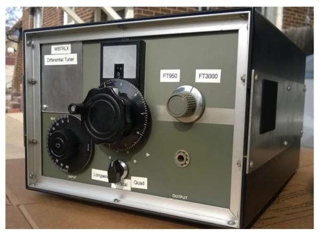
Figure 66: WB7RLX Differential Tuner – Note the unused hole in the front. I'm going to mount a propagation compensator in the unit and locate the control switch there. A note on the six position antenna selector switch: When the switch is pointing above horzontial, as it is in the picture, the tuner is engaged. If the arrow is pointing below the horzontial then the tuner is disengaged.
