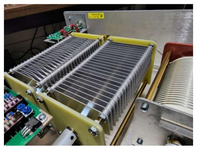
Figure 86: Palstar AT2K variable capacitors
