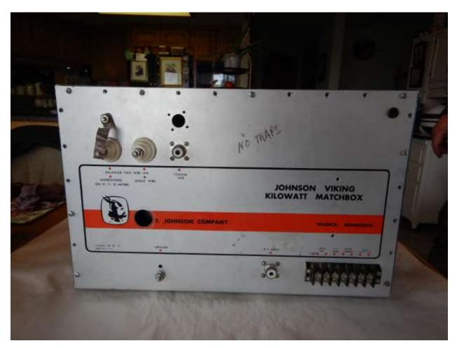
Figure 59: KW Johnson Matchbox - Rear view. Note the extra hole that someone added for an SO-239 socket. The small hole in the top right was for the SWR wire that attached to an external directional coupler.
