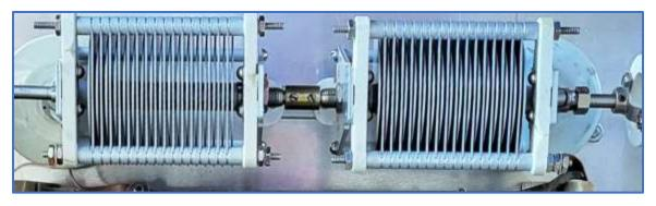
Figure 15: Variable Split Stator - Basically a split stator is two capacitors sharing a single shaft. You can wire the device to be two independent devices or connect the two capacitors together in series to increase the range of the device.
