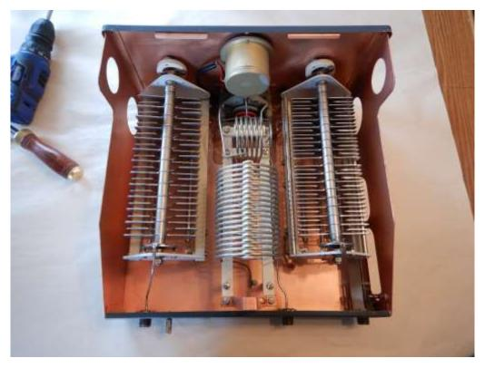
Figure 74: James Millen 92200 Ultimate Transmatch - The case is made completely of copper!
