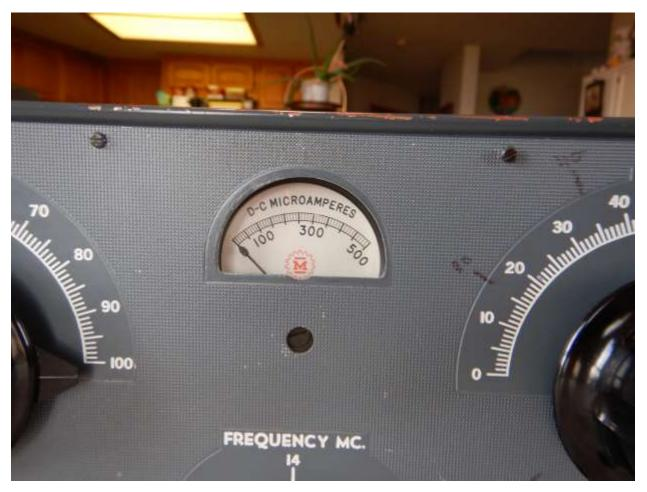
*Figure 79: James Millen 92200 Ultimate Transmatch – Power (SWR) Meter. A front panel switch was used to select forward or reflected power.*
