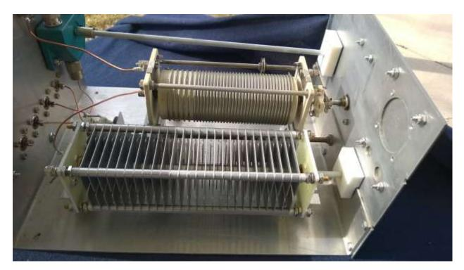
Figure 68: WB7RLX Differential Tuner – This is a good view of the differential capacitor that originally was in the MFJ-986 tuner. It does appear to be of good quality. It should also be fine for use with 600 watts or less. I'm afraid that if I were to put 1000 watts into the tuner with a high SWR I would get flash-over in the capacitor. Note also that the capacitor and inductor are isolated from the front panel.
