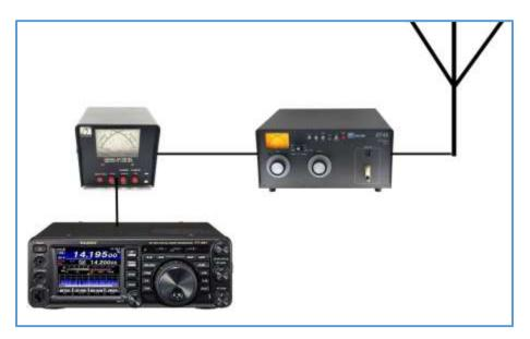
Figure 28: Typical Station Using an External Tuner
